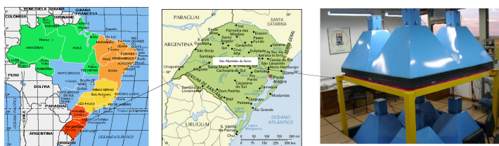
Figure 3 – The Ground Multi-Directional Cosmic Ray-Muon Detector installed at the Southern Space Observatory – SSO, in São Martinho da Serra, South of Brazil.
